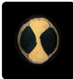
Press-fit geometry cross section (bow-tie)
