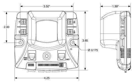
The MDL-BDC24 should be mounted so that the vents in the top and sides of the module are not restricted in any way. A clearance of  $\frac{1}{2}$  inch should be maintained around the module.
