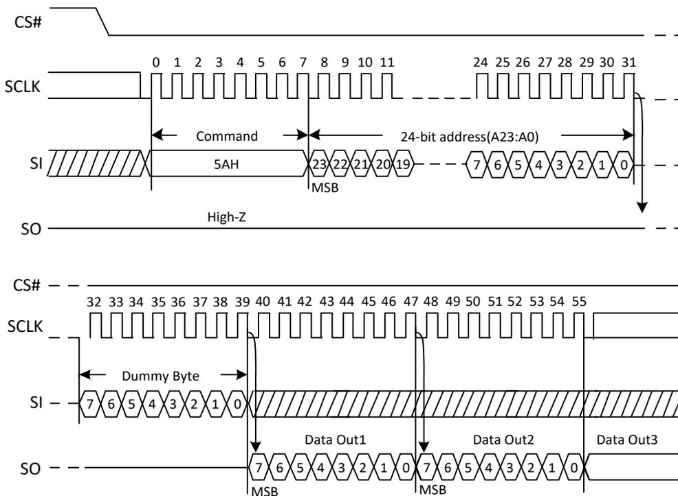
Note: A23-A8 = 0, A7-A0 is the starting byte address for 256-byte SFDP Register.
