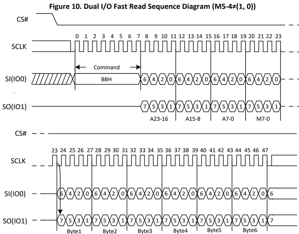
Figure 10a. Dual I/O Fast Read Sequence Diagram (M5-4= (1, 0))
