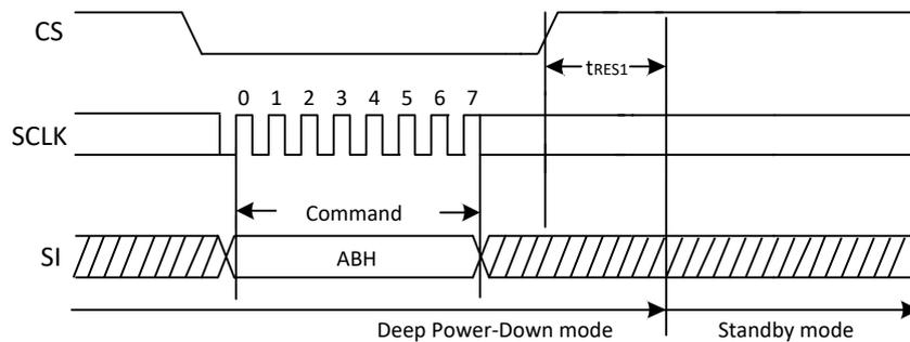
Figure 21a. Release Power-Down/Read Device ID Sequence Diagram
