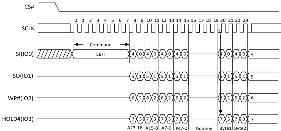
**Quad I/O Fast Read with “Continuous Read Mode”**
