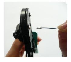
Remove the crimped contact.
