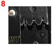
Close the tool lightly until the contact is held (1. Ratchet Lever)
