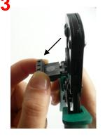
Click out the Flap locator stop. Schwenkanschlag herausklappen.
