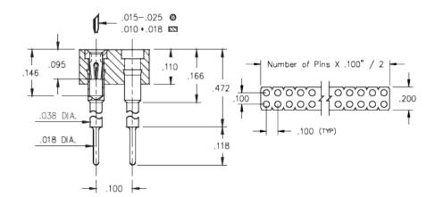
**Description:** Interconnect Socket Elevated Strip Socket Accepts .015"- .025" (0,38 - 0,635 mm) dia leads Double Row Through Hole Plating Code: Shell Plating: 200 μ" Tin/Lead(93/7) over 100 μ" Nickel Inner Contact Plating: 30 μ" Gold over 50 μ" Nickel
