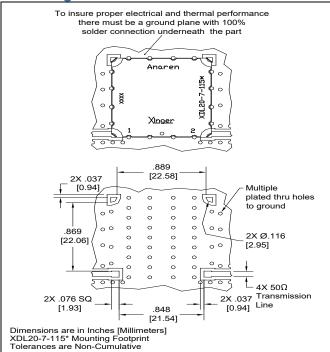
In order for Xinger surface mount delay lines to work optimally, there must be  $50\Omega$  transmission lines leading to and from all of the RF ports. Also, there must be a very good ground plane under the part with a number of plated thru holes to insure proper electrical performance. If any of these conditions are not satisfied, insertion loss, average delay and VSWR may not meet published specifications.
