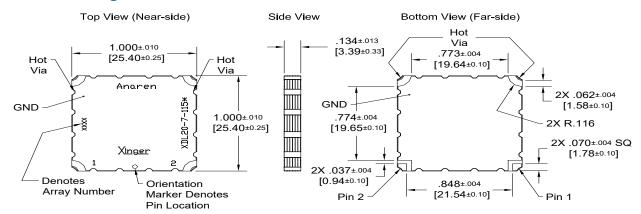
Dimensions are in Inches [Millimeters] XDL20-7-115\* Mechanical Outline
