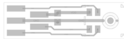
Figure 3. EV_ICS-40619-FX Board Layout (Top View) 12 mm x 3.6 mm
