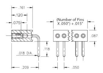
**Description:** Interconnect Socket Right Angle Socket Accepts .015" - .020" (0,38 - 0,508 mm) dia leads Single Row Through Hole Plating Code: **Shell Plating:** 200 μ" Tin (matte finish) over 100
