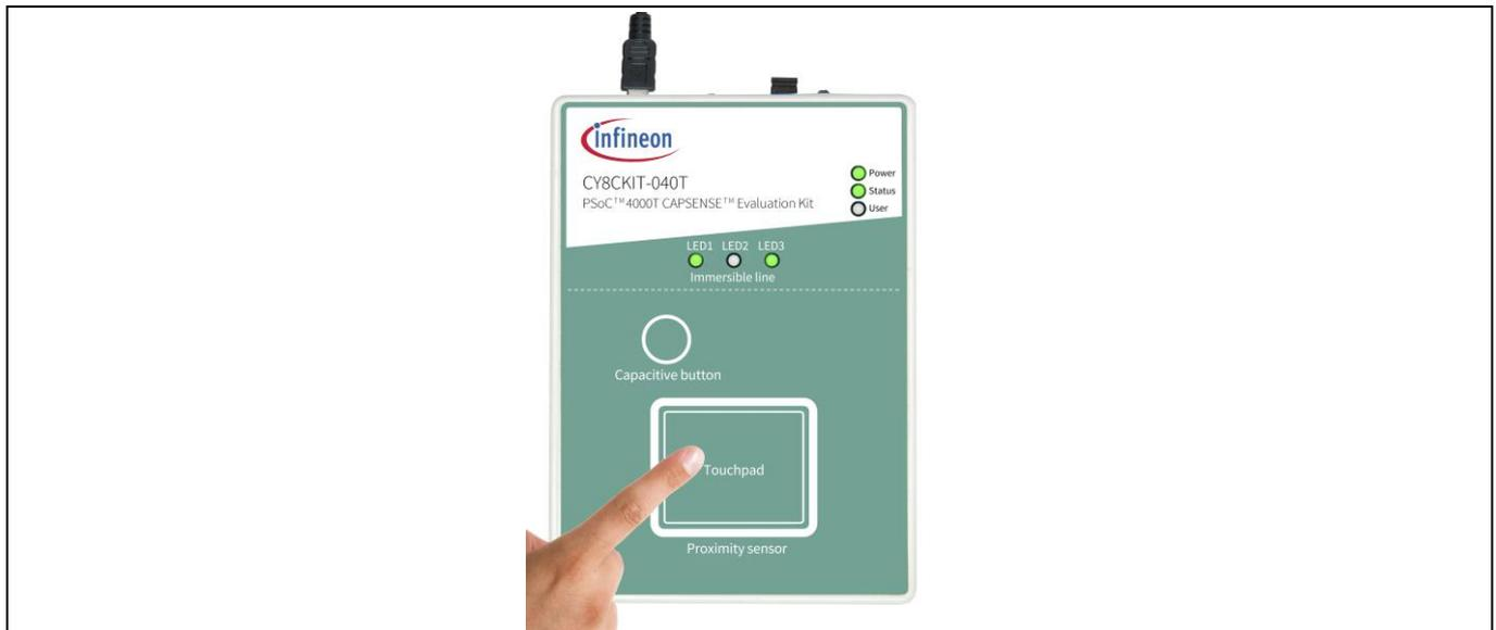
**Figure 7 Capacitive touchpad operation with LED indication**
