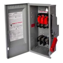
Siemens Low Voltage Circuit Protection Heavy Duty Safety Switches. Type: ENCLOSED, SAFETY SWITCH Std: UL V. Rating: 600V A. Rating: 60A Wattage: 4W No. Of Poles: 3P F. Rating: 60Hz Action: SINGLE THROW Material: STEEL Enclosure: TYPE 1. 2-3 point mounting holes. O. Cycles: 10000 O. Temperature: (-20F-120F) AMBIENT TEMPERATURE Environmental Conditions: INDOOR
