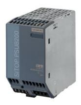
SITOP PSU8200 48 V/10 A Stabilized power supply input: 3 AC 400-500 V output: 48 V DC/10 A
