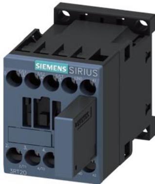
power contactor, AC-3 12 A, 5.5 kW / 400 V 1 NO, 24 V DC 0.85-1.85\*US with varistor plugged on 3-pole, size S00 screw terminal not expandable with auxiliary switch
