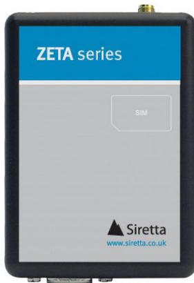
The ZETA-N-LTE (EU) is an industrial modem designed for regions of the world, where European frequencies are present. It will connect equipment to the 4G/LTE, 3G/UMTS & 2G / GSM cellular network. It has a 5 band LTE, dual band UMTS and dual band GPRS cellular engine, providing European frequency coverage.
