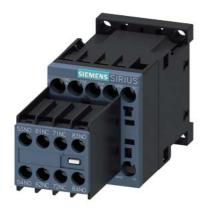
CONTACTOR RELAY, 4NO+4NC, AC 120V, 50/60 HZ, SIZE S00, SCREW TERMINAL, REMOVABLE AUX. SWITCH DIN EN 50005
