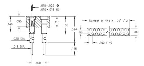
**Description:** Interconnect Socket Elevated Strip Socket Accepts .015"- .025" (0,38 - 0,635 mm) dia leads Double Row Through Hole Plating Code: **Shell Plating:**
