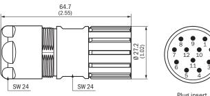
Plug insert 12 pin (plug-in face)
