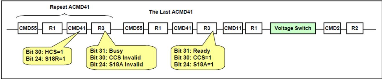
Figure 6-6-5 : ACMD41 Timing Followed by Voltage Switch Sequence
