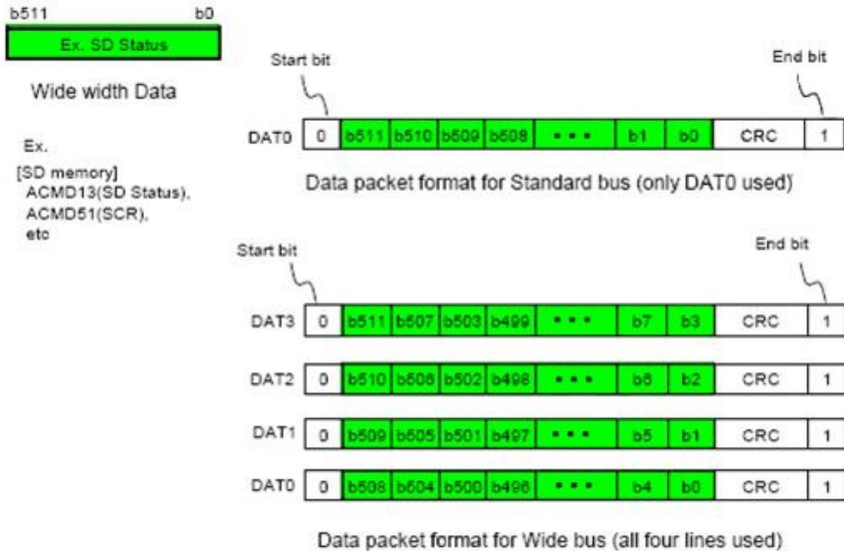
Figure 6-1-7: Data packet format - Wide width data
