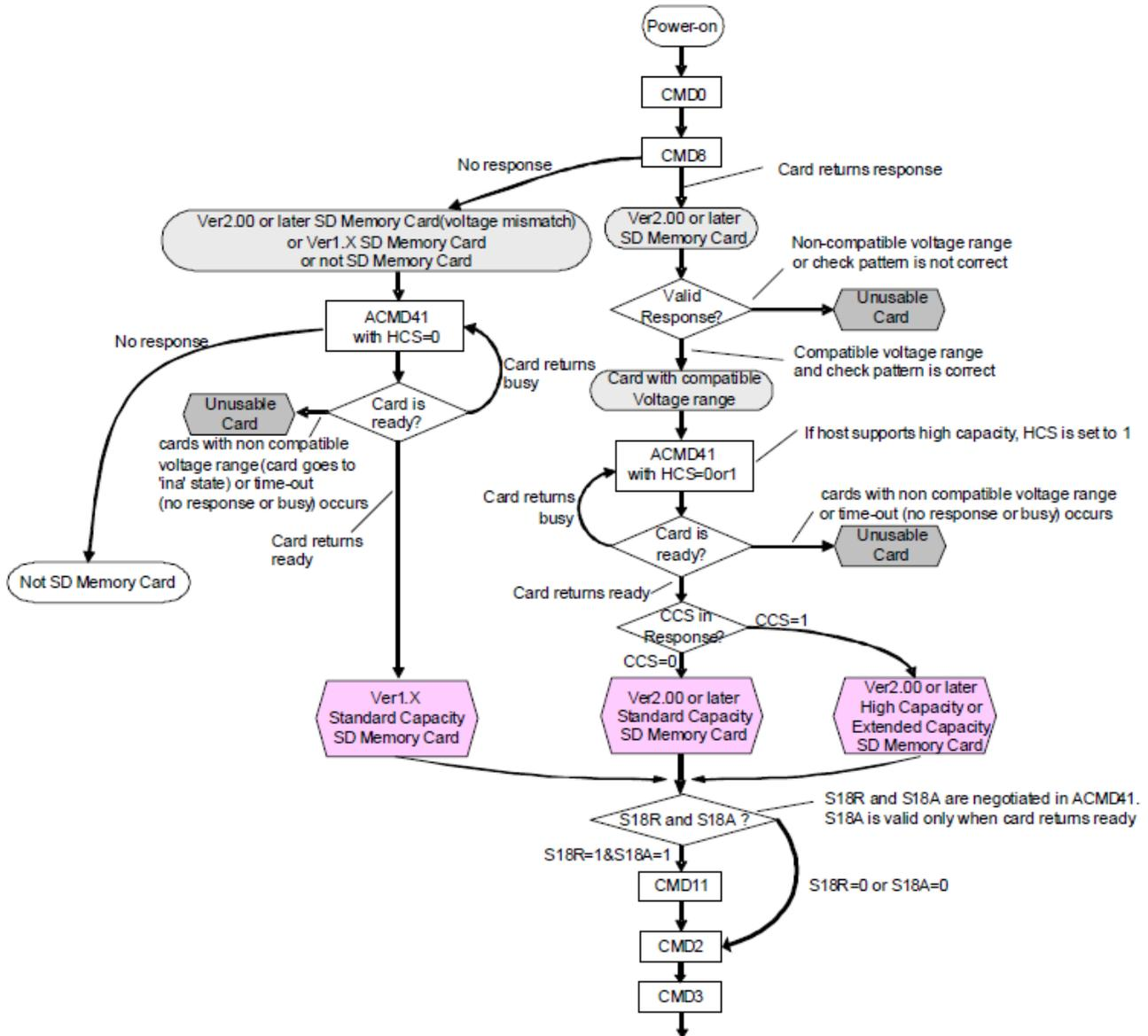
Figure 6-6-2: Card Initialization and Identification Flow (SD mode)
