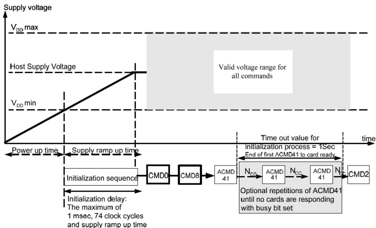
**Figure 2-1 Power-Up Diagram**
