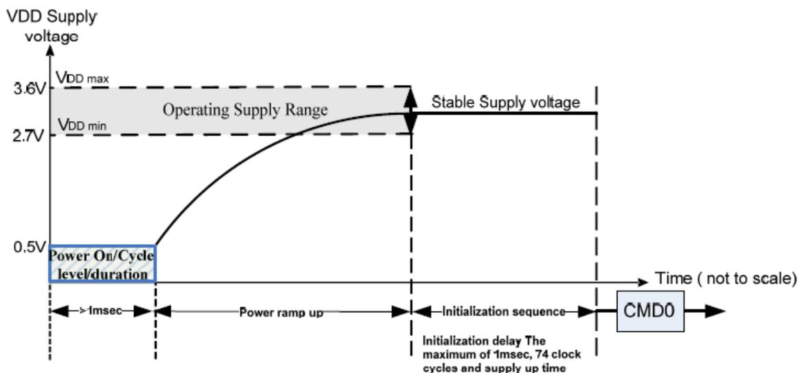
Figure 2-2 Change of Figure for power up
