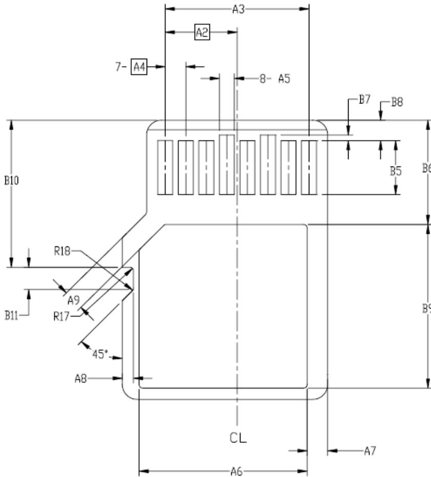
**Figure 3-15 -1 Dimensions of microSD (Bottom View)**
