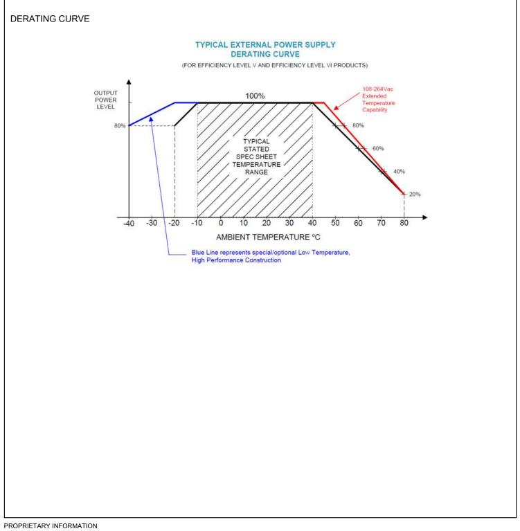
PROPRIETARY INFORMATION PROPRIETARY OF GLOBTEK, INC. ANY REPRODUCTION, DISCLOSURE OR USE OF THIS DRAWING, IN WHOLE OR IN PART, IS HEREBY PROHIBITED EXCEPT AS SPECIFIED IN WRITING BY GLOBTEK, INC. @ GlobTek, Inc. 2018 - 2024 Page 9 of 23
