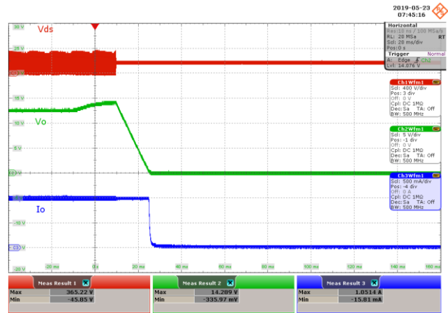
Figure 76 – 115 VAC 60 Hz. CH1: V_{DS} , 400 V / div., 20 ms / div. CH2: V_{OUT} , 5 V / div., 20 ms / div. CH3: I_{OUT} , 500 mA / div., 20 ms / div. V_{OUT(MAX)} = 14.289 V.
