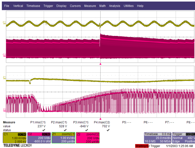
Figure 139 – DM Surge. V_{DS(MAX)} = 702 \text{ V} .
