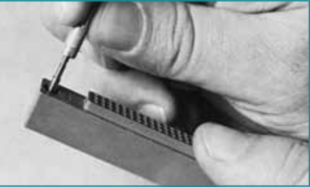
LOCKING SCREW ACCESSORY INSERTED INTO I/O CONNECTOR BODY
