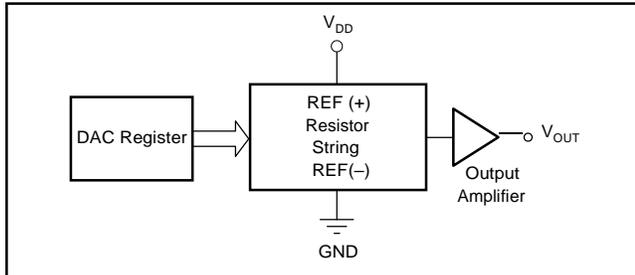
FIGURE 1. HT5320A Architecture.
