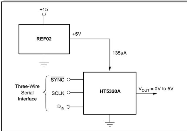
FIGURE 9. REF02 as Power Supply to HT5320A.
