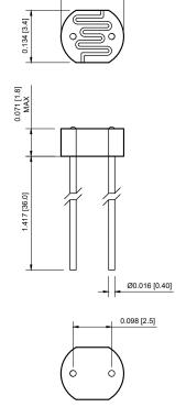
Note: Lead soldering temperature (1/16 inches away from body) 260°C for 3 sec.
