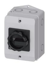
SENTRON, Switch disconnector 3LD, main switch, 3-pole, lu: 16 A, Operating power / at AC-23 A at 400 V: 7.5 kW, molded-plastic encapsulation for inch cable gland, 1 NC, 1 NO, rotary operating mechanism, black
