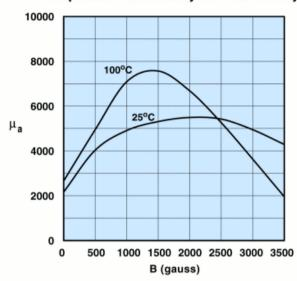
Measured on an 18/10/6mm toroid at 10kHz.
