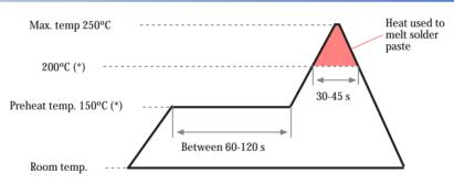
(\*) Melting point temp. depends on solder properties
