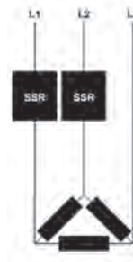
Two-phase SSR SOB to control heaters connected in delta (for high voltage, balanced or unbalanced loads)
