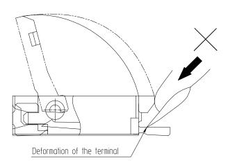
2. The actuator rotates around the rotational axis as shown below. Please rotate the actuator.
