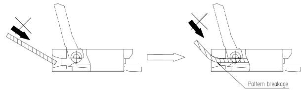
2. Do not insert the FPC diagonally from above If the FPC is inserted at a slat (incorrectly) as shown below in the FPC insertion process, the FPC may bend and patterns may break or the FPC may not insert completely. resulting in improper conduction.
