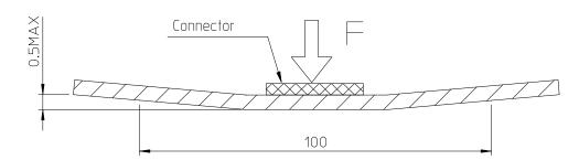
[INSTRUCTIONS ON INSERTING FFC/FPC AND CONNECTOR]
