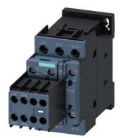
Power contactor, AC-3 38 A, 18.5 kW / 400 V 2 NO + 2 NC, 220 V AC 50/60 Hz, 3-pole Size S0, screw terminals Removable auxiliary switch
