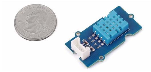
This temperature & humidity sensor provides a pre-calibrated digital output. A unique capacitive sensor element measures relative humidity and the temperature is measured by a negative temperature coefficient (NTC) thermistor. It has excellent reliability and long term stability. Please note that this sensor will not work for temperatures below 0 degree.
