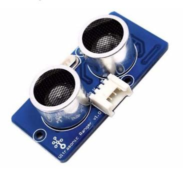
This Grove - Ultrasonic ranger is a non-contact distance measurement module which works at 40KHz. When we provide a pulse trigger signal with more than 10uS through singal pin, the Grove\_Ultrasonic\_Ranger will issue 8 cycles of 40kHz cycle level and detect the echo. The pulse width of the echo signal is proportional to the measured distance. Here is the formula: Distance = echo signal high time \* Sound speed (340M/S)/2. Grove\_Ultrasonic\_Ranger's trig and echo singal share 1 SIG pin.
