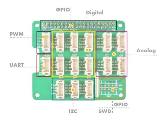
GPIO : The same pin out as the raspberry pi.
