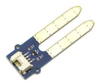
This Moisture Senor can be used for detecting the moisture of soil or judge if there is water around the sensor, let the plant in your garden able to reach out for human's help when they are thirsty. This sensor is very easy to use, you can just simply insert in into the soil and read the data. With this sensor, you can make a small project that can let the plant send a message to you like " I am thirsty now, please feed me some water."
