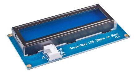
This Grove – 162 LCD module is a 16 Characters 2 Lines LCD display, it uses I2C bus interface to communicate with the development board, thus these will reduce the pin header from 10 to 2 which is very convenient for the Grove system. This LCD display module also supports customise characters, you can create and display heart symbol or stick-man on this LCD module through a simple coding configuration.
