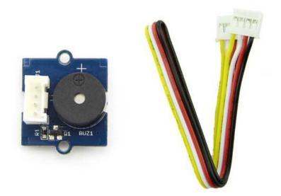
This module uses piezo buzzer as the main component, it can produce high pitch tone while it is connected to digital output and logic level set to High, otherwise it can produce various tones according to the frequencies generated from the Analog PWM output that connected to it. (note: the frequency range that normal human ear can distinguish is between 20 Hz and 20kHz.)
