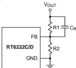
Figure 1. C<sub>ff</sub> Capacitor Setting
