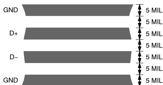
Figure 16. Arrangement of Signal Tracks
