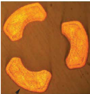
Au/Ni Barrier (Uniform plating thickness)
