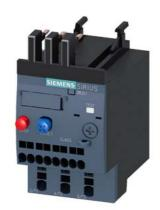
Overload relay 11...16 A Thermal For motor protection Size S00, Class 10 Contactor mounting Main circuit: Spring-type terminal Auxiliary circuit: spring-type terminal Manual-Automatic-Reset
