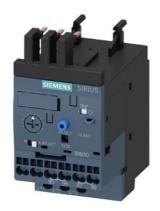
Overload relay 4...16 A Electronic For motor protection Size S00, Class 20E Contactor mounting Main circuit: Spring-type terminal Auxiliary circuit: Spring-type terminal Manual-Automatic-Reset
