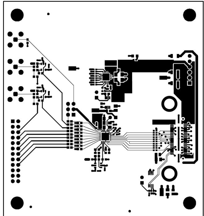
Figure 18. ADS8168 EVM PCB Layer 1: Top Layer
