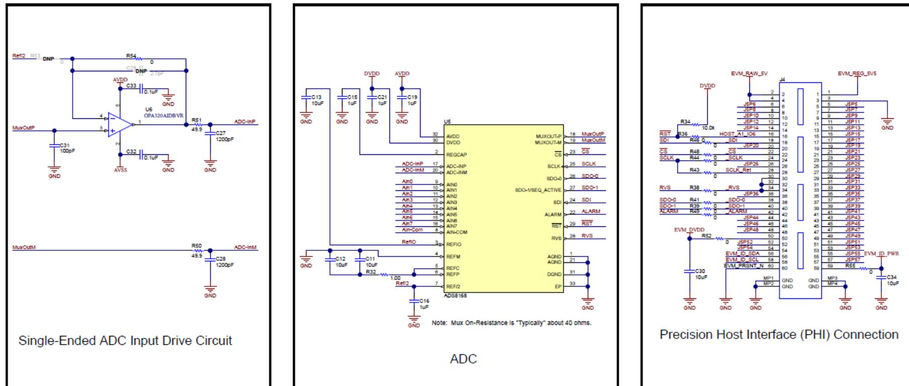
Figure 22. ADS8588EVM-PDK Schematic
