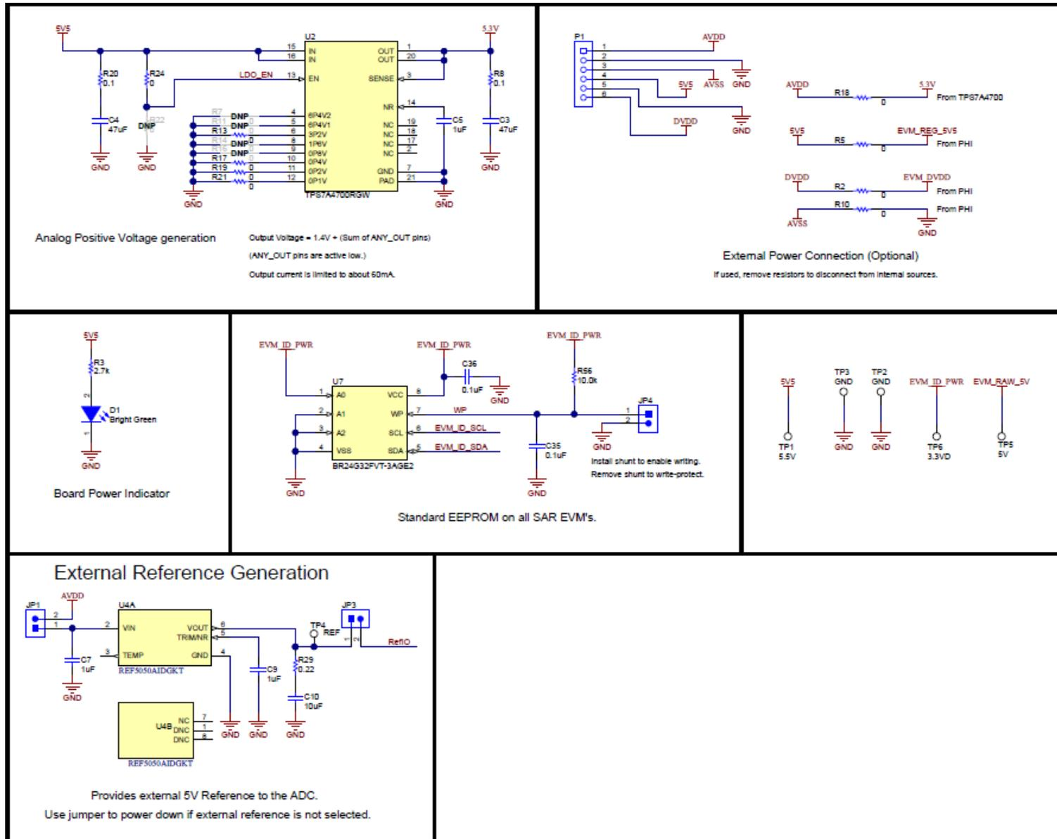
Figure 24. ADS8588EVM-PDK Schematic
