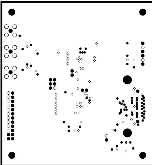
Figure 19. ADS8168 EVM PCB Layer 2: GND Plane
