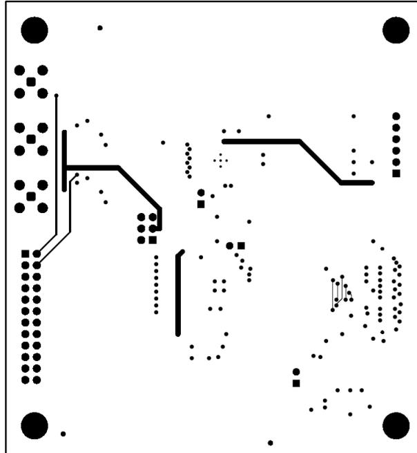
Figure 21. ADS8168 EVM PCB Layer 4: Bottom Layer
