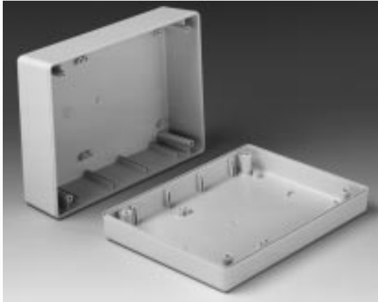
Battery compartment type of case size 155 for 1 flat battery 9 V (PP3) or 2 mignon-cells 1.5 V (AA). (Order contacts separately; see page 103)
