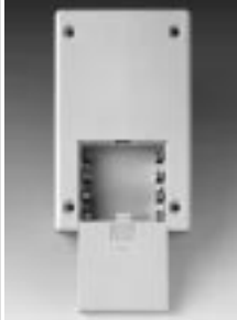
Battery compartment type of case sizes 155, 190 for 4 mignon-cells 1.5 V (AA) or 2 flat batteries 9 V (PP3). (Clips for AA cells fitted).
