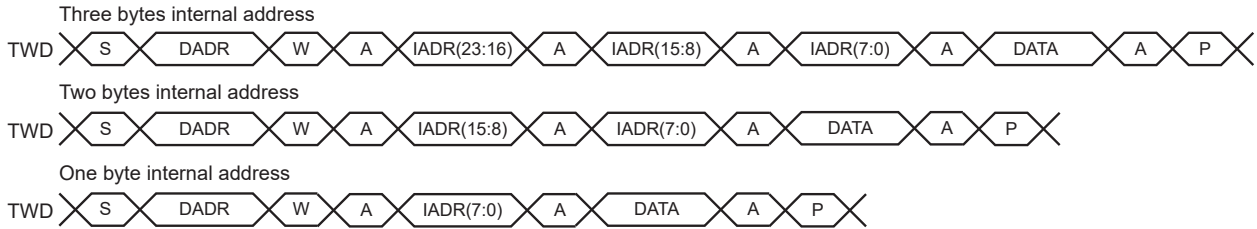
Figure 46-92. Host Write with One, Two or Three Bytes Internal Address and One Data Byte
