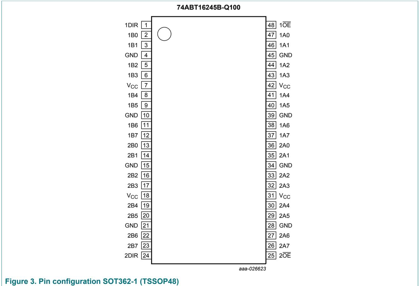
Figure 3. Pin configuration SOT362-1 (TSSOP48)
