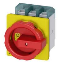
SENTRON, Switch disconnector 3LD, emergency switching-off switch, 3- pole, lu: 125 A, operating power / at AC-23 A 400 V: 45 kW, front-mounted, rotary operating mechanism, Red / yellow, 4-hole mounting of the handle
