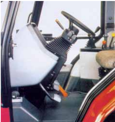
Picture 2.7: iglidur® G plain bearings have been proven in control levers and pedals of farm tractors and construction vehicles
