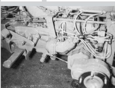
Picture 2.4: Vibrations, dirt, and temperatures up to 130°C occur in the area surrounding the engine
