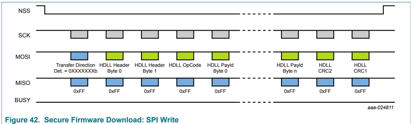
Figure 42. Secure Firmware Download: SPI Write
