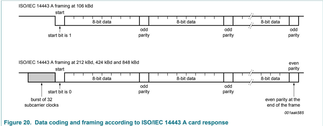
Figure 20. Data coding and framing according to ISO/IEC 14443 A card response
