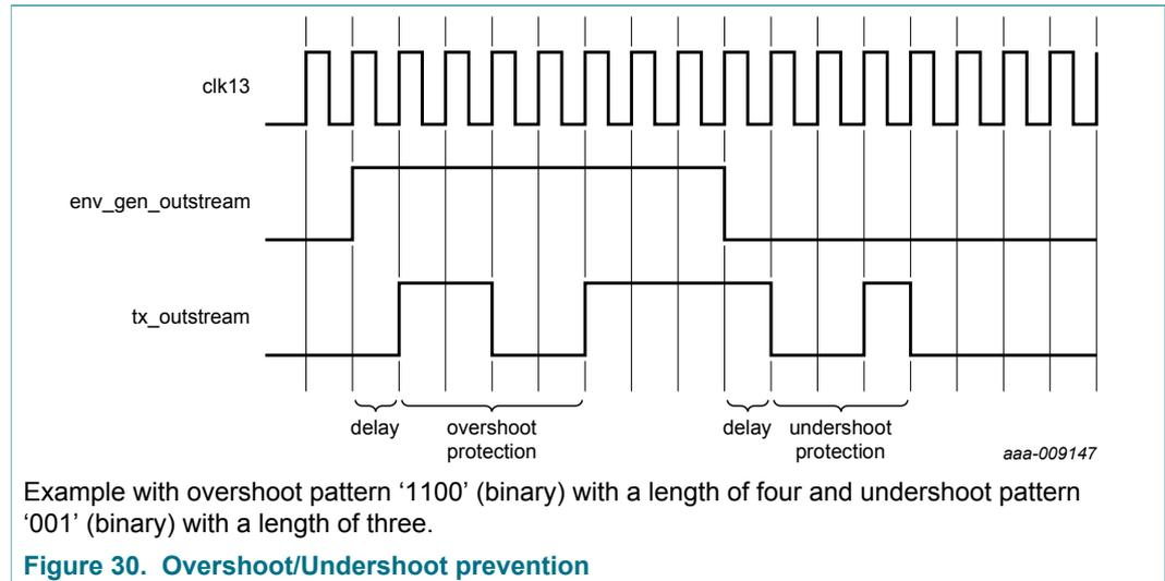
The over- and undershoot protection allows configuring additional signals on the Transmitter output which allows to control the signal shaping of the antenna output.
