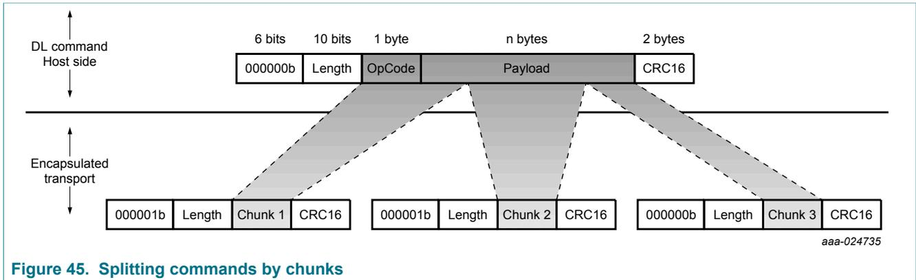
Figure 45. Splitting commands by chunks
