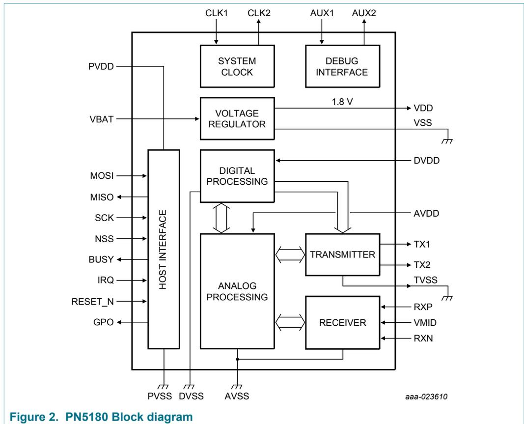
Figure 2. PN5180 Block diagram
