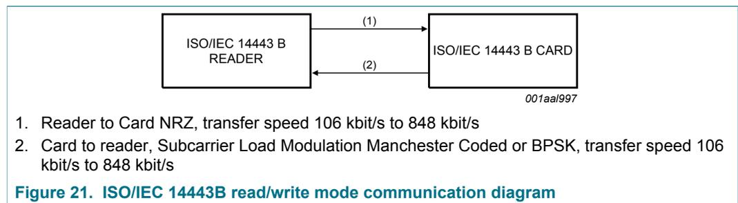
Figure 21. ISO/IEC 14443B read/write mode communication diagram
