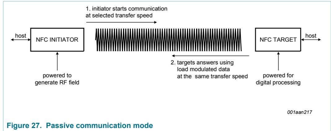
Figure 27. Passive communication mode
