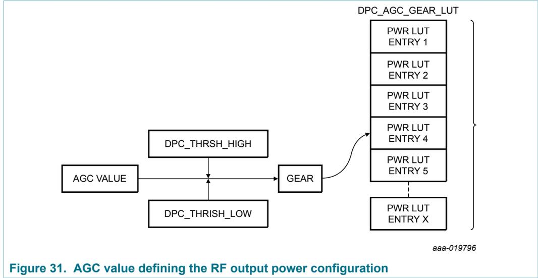
Figure 31. AGC value defining the RF output power configuration
