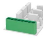
PCB headers, nominal current: 76 A, rated voltage (III/2): 1000 V, number of positions: 2, pitch: 10.16 mm, color: green, contact surface: Silver, mounting: Wave soldering, The nominal current of 76 A applies in connection with connectors from the PC 16 family. 41 A are reached in connection with PC 6 connectors (50 A in accordance with UL).
