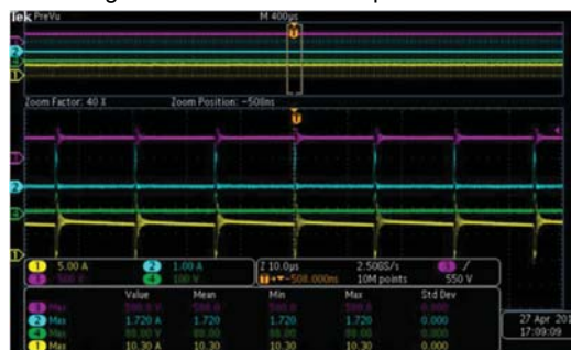
Figure 30. V_{IN}=264Vac Output Short
