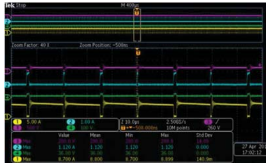
Figure 24. V_{IN}=90Vac Output Short
