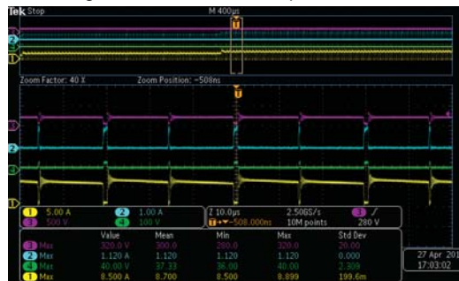
Figure 26. V_{IN}=115Vac Output Short
