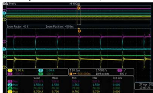
Figure 28. V_{IN}=230Vac Output Short
