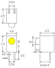
Dimensions : Millimetres Tolerance : ±0.25mm
