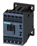
Power contactor, AC-3 16 A, 7.5 kW / 400 V 1 NC, 42 V AC, 50/60 Hz 3-pole, Size S00 Spring-type terminals
