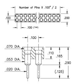
**Description:** Interconnect Flat Face Target Connector Spring-Loaded Header Vertical Mount Through Hole Target Double Row Through Hole Plating Code: Shell Plating: 10 μ" Gold over 100 μ" Nickel Packaging: Packaged in Bulk
