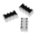
The MRS series is an entirely new chip network utilising nickel chrome sputtering on high purity alumina. This network has been designed for high volume applications and is offered with 4 isolated resistors on a single substrate (12.06 sizes) at 0.1% with convex terminals. A wide value range and alternative T.C.R's make this a most versatile resistor solution.
