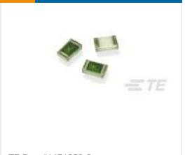
TE Part #1676298-2 RN 0805 301R 0.1% 10PPM 1KRL
