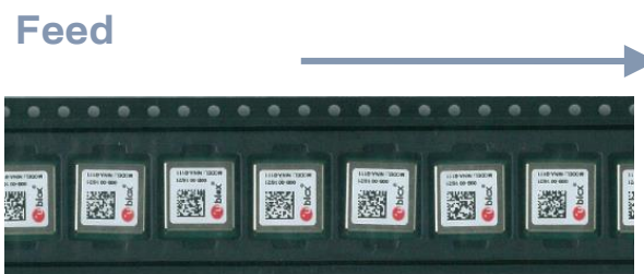
Figure 12: Orientation of NINA-B111 modules on tape
