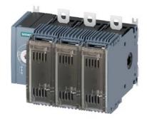
Switch disconnector with fuse 160 A, Size 2, 3-pole for LV HRC fuse Sz. 000 and 00 Front operating mechanism left Basic unit without handle flat terminal
